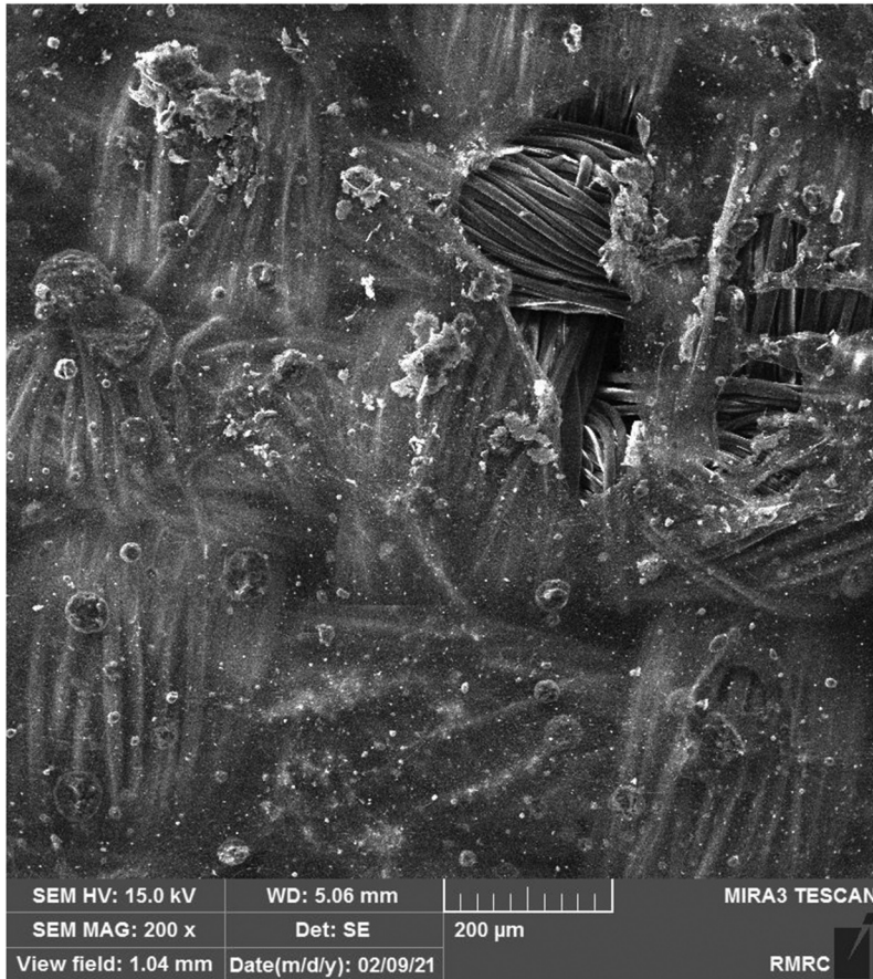
Figure 6. FESEM image of palm cellulose\CMN layer electrospun on viscose fabric.
